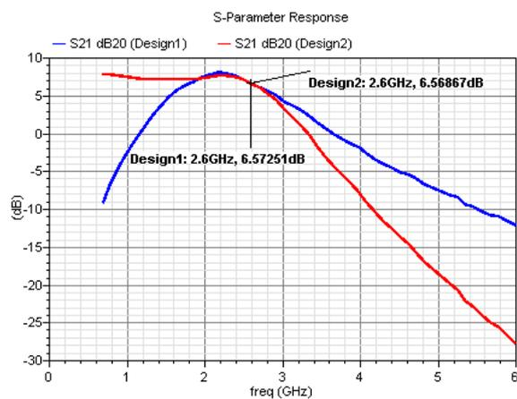
Figure 7. S21 plot (in dB) versus frequency
